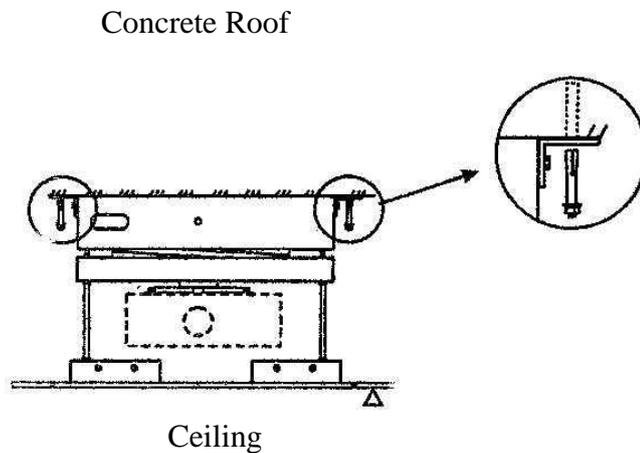
3. Open the ceiling 3CM larger each side than size of this projector lift's chassis.
